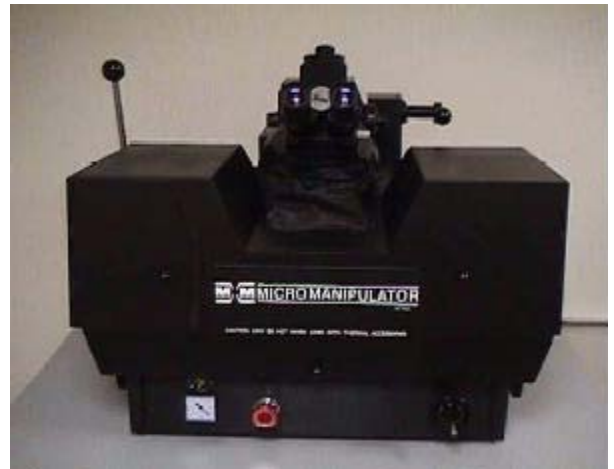
Closed 8800-ISE provides electrical and light shielding
