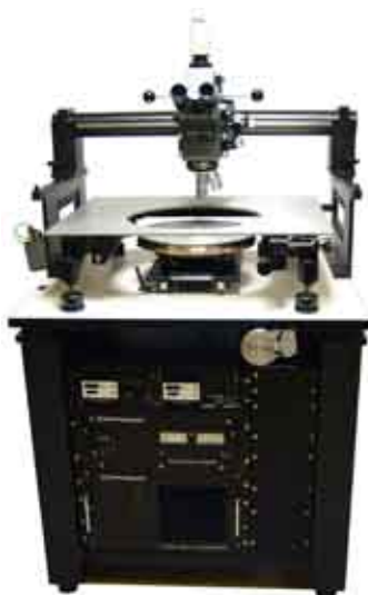
Figure 5 A 2200-WLR Probe Station
