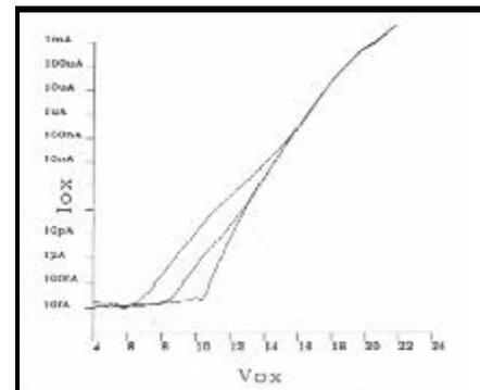
**Figure three.** A typical Time Dependent Dielectric Leakage curve family derived from circuit b in figure one.
