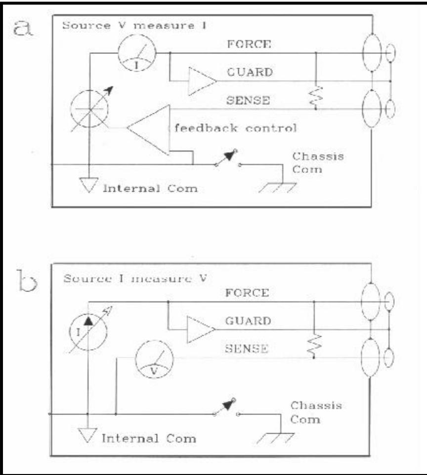
**Figure four.** The two generalized basic configurations for Source Measure Units. (a): Source V, measure I. (b): Source I, measure V.
