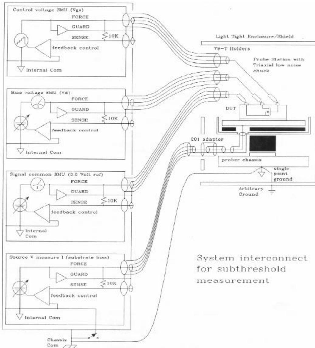
System interconnect for subthreshold measurement
