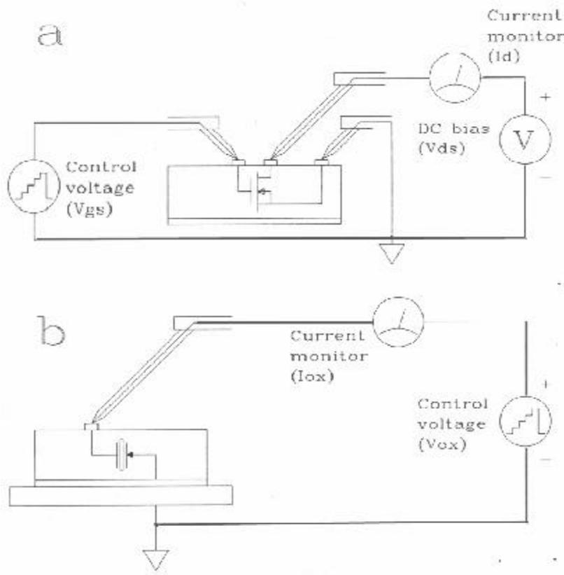
**Figure One:** Idealized representations of surface to surface and surface to substrate current measurements for (a): MOSFET subthreshold characterization. (b): Time Dependent Dielectric Leakage characterization. Grounding and shielding requirements and practical SMU connections.
